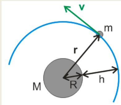
$$\text{Kreisbewegung} \rightarrow \left. \begin{aligned} m \frac{v^2}{r} &= G \frac{Mm}{r^2} \\ r &= R + h \end{aligned} \right| \rightarrow v^2 = G \frac{M}{R+h} = \frac{gR^2}{R+h}$$
